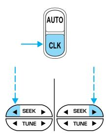
To set the minute, press and hold the CLK control and press TUNE:
